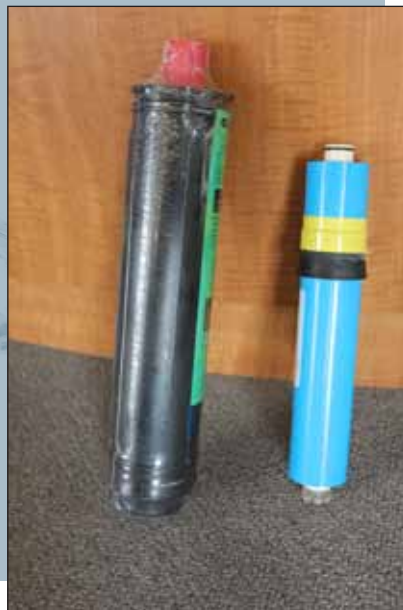
Reverse osmosis membranes
